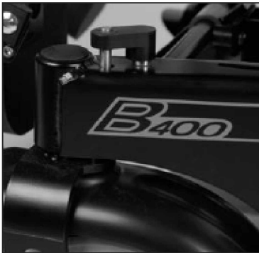
Mechanical swivel lock
